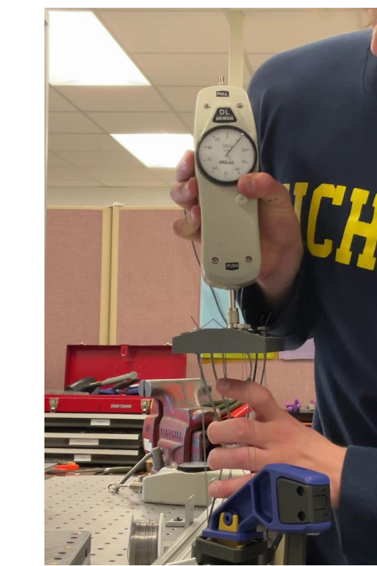
Axial test measured similar loads for the different buckling presets
